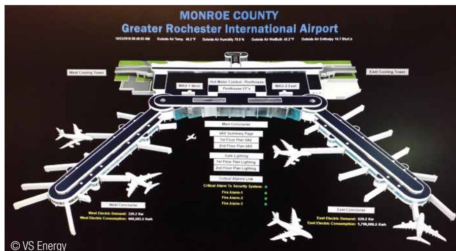
Main Alerton Graphic Screen for the Greater Rochester International Airport
